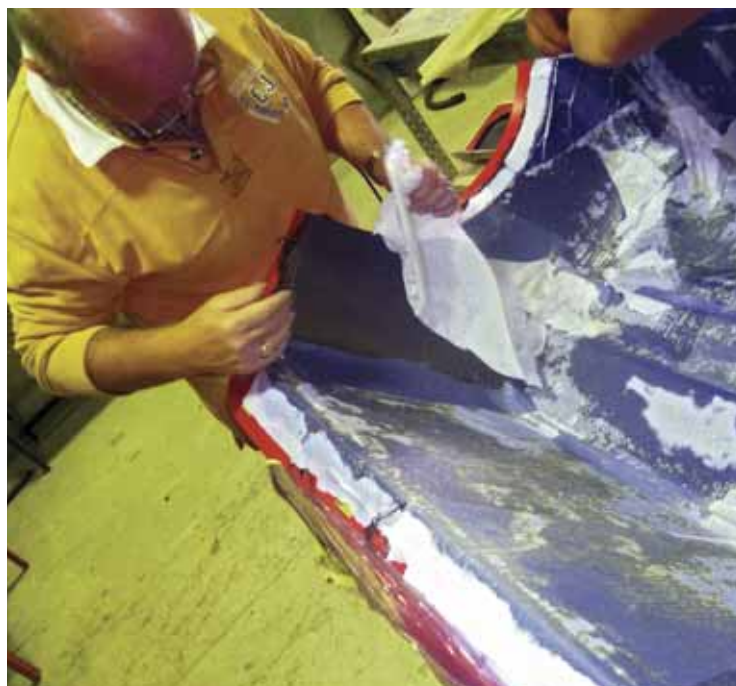
Lower left - Peel ply was used to ensure all parts were smooth on the inside as well as on the outside, attention to detail is very important in this industry.
